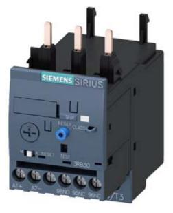
Overload relay 6...25 A for motor protection size S0, CLASS 10E contactor mounting Main circuit: screw term. Aux. circuit: screw term. Manual/Auto RESET
