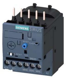
Overload relay 3...12 A for motor protection size S00, CLASS 10E contactor mounting Main circuit: screw term. Aux. circuit: screw term. Manual/Auto RESET
