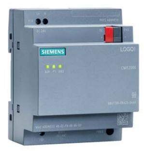
LOGO! CMK2000 COMMUNICATION MODULE TO INTEGRATE THE LOGO! 8 IN THE BUILDING BUS KNX POWER SUPPLY DC 24V 0,04A 1 RJ45 PORT FOR ETHERNET CONECTION 50 COMMUNICATION OBJECTS TIME SYNCHRONISATION CONFIG./DIAG.PER WEB-INTERFACE
