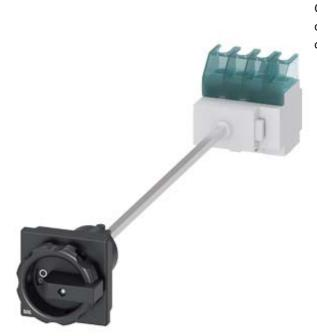
SENTRON, 3LD switch disconnector, main switch, 4- pole, lu:25 A, Operational power / at AC-23 A at 400 V: 9,5 kW, floor mounting with door coupling, rotary operating mechanism, black, 4- hole mounting of the handle
