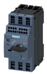
CIRCUIT-BREAKER SZ S00, FOR MOTOR PROTECTION, CLASS 10, A-REL. 0.55...0.8A, N-RELEASE10A, SPRING-L. CONNECTION STANDARD SW. CAPACITY W. TRANSVERSE AUX. SWITCH 1NO+1NC
