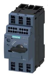
CIRCUIT-BREAKER SZ S00, FOR MOTOR PROTECTION, CLASS 10, A-REL. 0.18...0.25A, N-RELEASE3.3A SPRING-L. CONNECTION STANDARD SW. CAPACITY W. TRANSVERSE AUX. SWITCH 1NO+1NC
