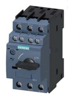
CIRCUIT-BREAKER SZ S0, FOR MOTOR PROTECTION, CLASS 10, A-RELEASE 16...22A, N-RELEASE 286A, SCREW CONNECTION, STANDARD SW. CAPACITY, W. TRANSVERSE AUX. SWITCH 1NO+1NC
