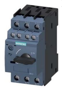
CIRCUIT-BREAKER SZ S0, FOR MOTOR PROTECTION, CLASS 10, A-RELEASE 30...36A, N-RELEASE 432A, SCREW CONNECTION, STANDARD SW. CAPACITY, W. TRANSVERSE AUX. SWITCH 1NO+1NC
