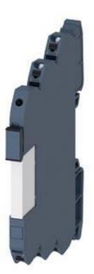
Output coupler with plug-in relay, 1 CO Spring-type terminal (push-in) 230 V AC/DC Enclosure width 6.2 mm Thermal current 6 A
