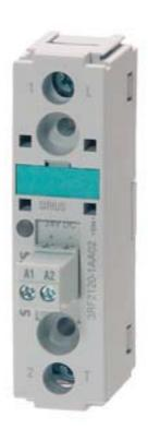
SEMICONDUCTOR RELAY 3RF2, 1-PH. WIDTH 22.5MM, 30 A 48-460 V / 110-230 V AC SCREW TERMINAL
