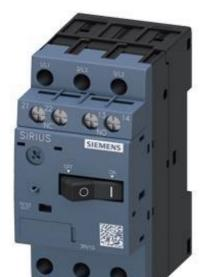
CIRCUIT-BREAKER, SIZE S00, FOR MOTOR PROTECTION, CLASS 10, A REL.0.11...0.16A, N REL.2.1A SCREW CONNECTION, STANDARD BREAKING CAPACITY, W. TRANSV. AUX. SWITCH 1NO/1NC
