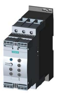
SIRIUS SOFT STARTER, S2, 72A, 37KW/400V, 40 DEGR., AC 200-480V, AC/DC 110-230V, SPRING-LOADED TERMINALS
