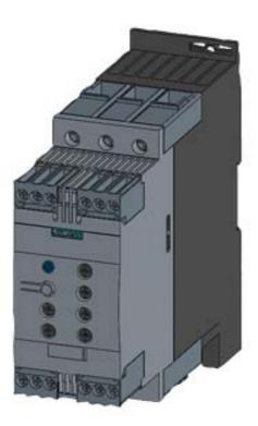
SIRIUS SOFT STARTER, S2, 45A, 22KW/400V, 40 DEGR., AC 200-480V, AC/DC 24V, SCREW TERMINALS, THERMISTOR MOTOR PROTECTION
