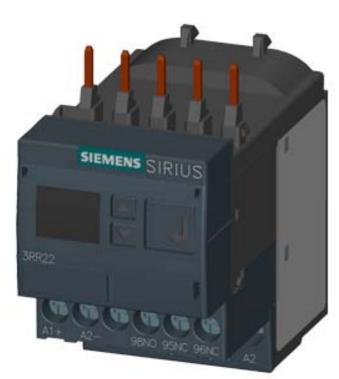
MONITORING RELAY ATTACHABLE TO CONTACTOR 3RT2. SIZE S00 STANDARD, DIGITAL ADJUSTABLE APPARENT/ACTIVE CURRENT MONIT. 1.6 - 16A, 20-400 HZ, 3-PHASE SUPPLY 24 V AC/DC 1 CO CONTACT, 1 SEMICOND. OUTPUT FOR ALARM AND WARNING, MONITORING FOR CURRENT OVERSHOOT/UNDERSHOOT PHASE FAILURE, WIRE BREAK PHASE SEQUENCE FAULT CURRENT BLOCKING CURRENT WARNING AND ALARM THRESHOLDS WITH OR W/O ERROR LOG ON-DELAY 0-99 S SPURIOUS PEAK SUPPR.0-30 S BREAK AFTER FAULT 0-300 MIN SCREW CONNECTION
