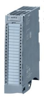
SIMATIC S7-1500, ANALOG INPUT MODULE AI 8 X U/I HF, 16 BITS OF RESOLUTION, ACCURACY 0.1%, 8 CHANNELS IN GROUPS OF 1; COMMON MODE VOLTAGE: 30V AC/60V DC, DIAGNOSIS, PROCESSALARMS; SCALABLE MEASURED VALUES, ADJUSTMENT OF MEASURING RANGE, CALIBRATION AT RUN INCL. INFEED ELEMENT, SHIELD CLAMP AND SHIELD **TERMINAL**
