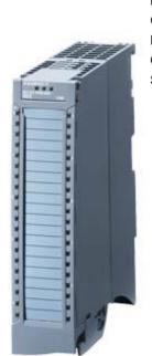
SIMATIC S7-1500, ANALOG INPUT MODULE AI 8 X U/I HS, 16 BITS OF RESOLUTION, ACCURACY 0.3 %; 8 CHANNELS IN GROUPS OF 8; COMMON MODE VOLTAGE APPR. 10V; DIAGNOSIS, PROCESSALARMS; 8 CHANNELS IN 0.0625 MS OVERSAMPLING INCL. INFEED ELEMENT, SHIELD CLAMP AND SHIELD TERMINAL
