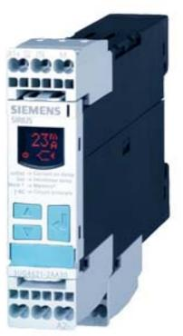
DIGITAL MONITORING RELAY CURRENT MONITORING, 22.5MM FROM 2 TO 500MA AC/DC OVERSHOOT AND UNDERSHOOT SUPPLY VOLTAGE: AC/DC 24V DC AND AC 50 TO 60 HZ NO GALVANIC ISOLATION FROM MEASURING CIRCUIT STARTUP AND INTERF. PEAK DELAY 0.1 TO 20S HYSTERESIS 0.1 TO 250MA 1 CO CONTACT W. OR W/O ERROR LOG AUTOM. RESET SPRING-LOADED CONNECTION
