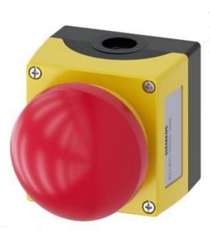
ENCLOSURE FOR COMMAND DEVICES, 22MM, ROUND, ENCLOSURE MATERIAL PLASTIC, ENCLOSURE TOP PART YELLOW, 1 COMMAND POINT PLASTIC, COMMAND POINT AT CENTER, A=EM. STOP PALM PUSHBUTTON RED, POSITIVE LATCHING, PULL TO UNLATCH, 1NC, 1NO, SCREW TERMINAL, BASE MOUNTING
