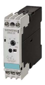
TIMING RELAY, SOLID-STATE, OFF-DELAY, 1 CO CONTACT, W/O AUX.VOLTAGE, 9 TIME SETTING RANGES 0.05S...600S, 200...240V AC/DC, WITH LED, SCREW TERMINAL
