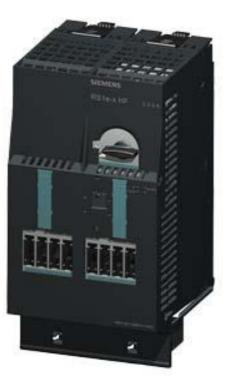
F-RS1E-X FOR ET 200S FAILSAFE REVERSING STARTER SETTING RANGE 2.4...8A MECHANICAL SWITCHING ELECTRONIC PROTECTION AC-3/TO 3KW/400V EXPANDABLE FOR BRAKE CONTROL MODULE 2DI MODULE 2DI MODULE SIGNAL FROM CIRCUIT-BREAKER PARAMETERIZABLE
