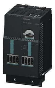
F-RS1E-X FOR ET 200S FAILSAFE REVERSING STARTER SETTING RANGE 2.4...16A MECHANICAL SWITCHING ELECTRONIC PROTECTION AC-3/TO 7.5KW/400V EXPANDABLE FOR BRAKE CONTROL MODULE 2DI MODULE 2DI CONTROL MODULE SIGNAL FROM CIRCUIT-BREAKER PARAMETERIZABLE
