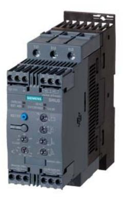
SIRIUS SOFT STARTER, S2, 72A, 37KW/400V, 40 DEGR., AC 200-480V, AC/DC 24V, SCREW TERMINALS, THERMISTOR MOTOR PROTECTION
