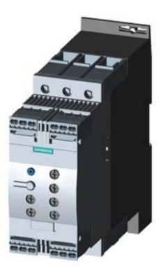
SIRIUS SOFT STARTER, S2, 72A, 37KW/400V, 40 DEGR., AC 200-480V, AC/DC 24V, SPRING-LOADED TERMINALS, THERMISTOR MOTOR PROTECTION
