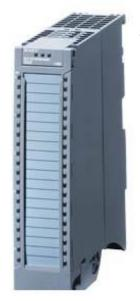
SIMATIC S7-1500, ANALOG OUTPUT MODULE AQ 8 X U/I HS 16 BITS OF RESOLUTION, ACCURACY 0.3 %, 8CHANNELS IN GROUPS OF 8, DIAGNOSIS, SUBSTITUTE VALUE 8 CHANNELS IN 0.125 MS INCL. INFEED ELEMENT, SHIELD CLAMP AND SHIELD TERMINAL
