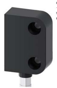
MAGNETICALLY OPERATED SWITCH, CONT. BLOCK, RECTANGULAR SMALL 26X36 MM, FOR DOOR HINGE LEFT, CONTACTS: SAFETY CONTACTS 2NC, SIGNALING CONTACT 1NC, WITH 8MM CATCH CONNECTION, CONNECTOR 6-POLE, WITHOUT LED, MATCHING SWITCHING MAGNET 3SE6714-3CA OR OFFSET BY 90 DEGREES 3SE6724-3CA
