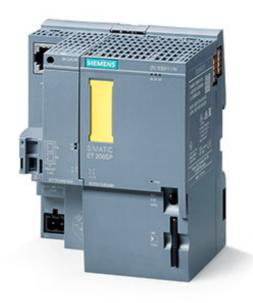
SIMATIC S7-1500, CPU 1511-1 PN, CENTRAL PROCESSING UNIT WITH WORKING MEMORY 150 KB FOR PROGRAM AND 1 MB FOR DATA, 1. INTERFACE: PROFINET IRT WITH 2 PORT SWITCH, 60 NS BIT-PERFORMANCE, SIMATIC MEMORY CARD NECESSARY
