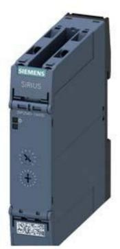
TIMING RELAY, ELECTRONIC, OFF-DELAY, WITHOUT CONTROL SIGNAL OR NON-VOLATILE RELAY DEFINITE PASSING MAKE CONTACT, 7 T. SET. RANGES 0.05S...600S, 12-240 V AC/DC, 1 CO CONTACT AT 50/60HZ AC W. LED, SCREW TERMINAL
