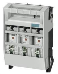
FUSE-SWITCH-DISCONNECTOR I = 160 A, U = 690 V, FOR SURFACE MOUNTING AND INSTALL., FLAT PAD CONNECTION M8, FUSE SIZE NH00
