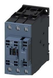
CONTACTOR,AC3:22KW/400V, 1NO+1NC, 20-33VAC/DC, COM.CAP. WITH VARISTOR, 3-POLE, SIZE S2, SPRING-TYPE TERMINAL
