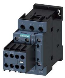
CONTACTOR, AC-3, 4KW/400V, 2NO+2NC, AC 230V 50HZ, 3-POLE, SZ S0 SCREW TERMINAL REMOVABLE AUX. SWITCH
