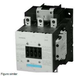
CONTACTOR, 275A/AC-1, AC(40...60HZ)/DC OPERATION UC 220...240V AUXIL. CONTACTS 2NO+2NC 3-POLE, SIZE S6 BAR CONNECTIONS CONVENT. OPERATING MECHANISM
