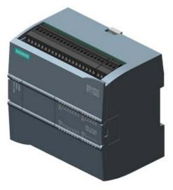
SIMATIC S7-1200, CPU 1214C, COMPACT CPU, AC/DC/RLY, ONBOARD I/O: 14 DI 24V DC; 10 DO RELAY 2A; 2 AI 0 - 10V DC, POWER SUPPLY: AC 85 - 264 V AC AT 47 - 63 HZ,
