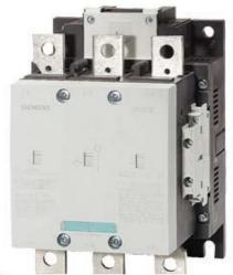
VAC. CONTACTOR, 132KW/400V/AC-3 AC(40...60HZ)/DC OPERATION UC 220-240V AUXILIARY CONTACTS 2NO+2NC 3-POLE, SIZE S10 BAR CONNECTIONS CONVENT. OPERATING MECHANISM
