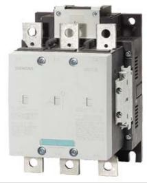
VAC. CONTACTOR, 110KW/400V/AC-3 AC(40...60HZ)/DC OPERATION UC 220-240V AUXILIARY CONTACTS 2NO+2NC 3-POLE, SIZE S10 BAR CONNECTIONS CONVENT. OPERATING MECHANISM
