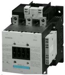
CONTACTOR, 90KW/400V/AC-3 AC(40...60HZ)/DC OPERATION UC 220-240V AUXILIARY CONTACTS 2NO+2NC 3-POLE, SIZE S6 BAR CONNECTIONS CONVENT. OPERATING MECHANISM CAGE CLAMP TERMINAL
