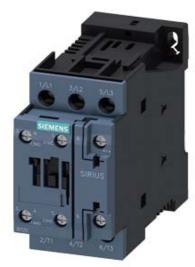
CONTACTOR, AC-3, 7.5KW/400V, 1NO+1NC, DC 24V, W.INTEGR.DIODE 3-POLE, SZ S0 SCREW TERMINAL
