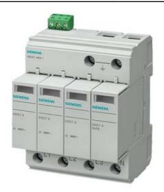
SURGE ARRESTER TYPE 2 REQUIREMENT CATEGORY C, UC 350V PLUG-IN PROTECTION BLOCKS 4POLE, 3+1 CIRCUIT FOR TN-S AND TT SYSTEMS W. REMOTE DISPLAY
