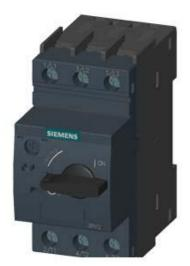
CIRCUIT-BREAKER SZ S0, FOR MOTOR PROTECTION, CLASS 10, A-REL.1.1...1.6A, N-REL.21A SCREW CONNECTION, STANDARD SW. CAPACITY
