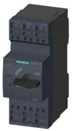
CIRCUIT-BREAKER SZ S0, FOR MOTOR PROTECTION, CLASS 10, A-RELEASE 27...32A, N-RELEASE 400A, SPRING-L. CONNECTION, STANDARD SW. CAPACITY,
