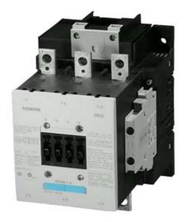
CONTACTOR, 90KW/400V/AC-3, AC(40...60HZ)/DC OPERATION UC 110...127V AUXIL. CONTACTS 2NO+2NC 3-POLE, SIZE S6 BAR CONNECTIONS CONVENTION. OPERATING MECHANISM SCREW TERMINAL
