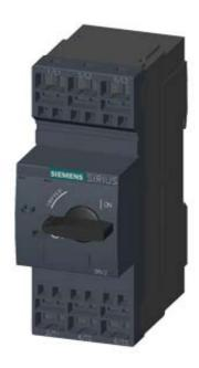
CIRCUIT-BREAKER SZ S0, FOR MOTOR PROTECTION, CLASS 10, A-RELEASE 18...25A, N-RELEASE 325A, SPRING-L. CONNECTION, STANDARD SW. CAPACITY,
