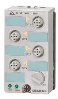
AS-INTERFACE COMPACT MOD. K45, IP67, DIGITAL, 4 OUTPUTS, 4 X OUTP., ELECTR.,1.0A, DC 24V 3AMAX. FOR ALL OUTPUTS 4 X M12 SOCKET
