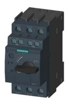
CIRCUIT-BREAKER SZ S00, FOR MOTOR PROTECTION, CLASS 10, A-REL. 0.7...1A, N-RELEASE 13A, SCREW CONNECTION, STANDARD SW. CAPACITY, W. TRANSVERSE AUX. SWITCH 1NO+1NC
