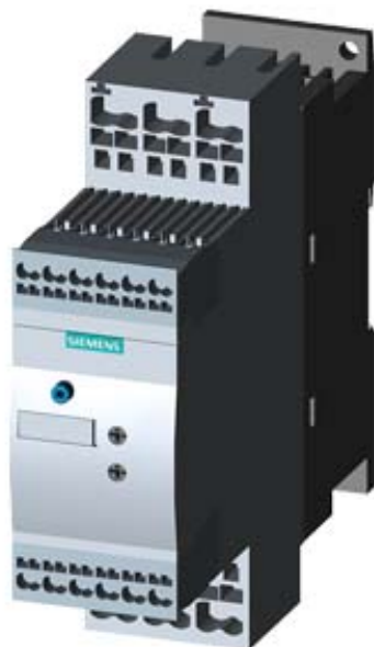
SIRIUS SOFT STARTER, SIZE S0, 32A, 15KW/400V, 40 DEGREES, 200-480V AC, 24V AC/DC, SPRING-LOADED TERMINALS
