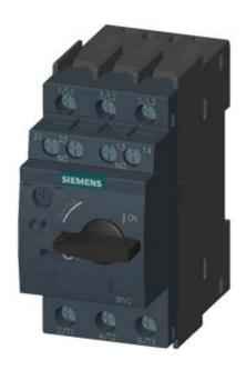
CIRCUIT-BREAKER SZ S0, FOR MOTOR PROTECTION, CLASS 10, A-RELEASE 23...28A, N-RELEASE 364A, SCREW CONNECTION, STANDARD SW. CAPACITY, W. TRANSVERSE AUX. SWITCH 1NO+1NC
