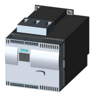
SIRIUS SOFT STARTER, VALUES WITH 400 V, 40 DEG., STANDARD: 93A, 45KW, INSIDE-DELTA CIRCUIT 3: 161A, 90KW, 200-460 V AC, 230 V AC, CAGE CLAMP TERMINALS
