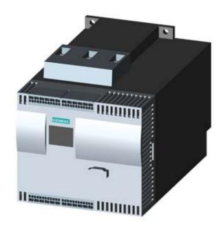
SIRIUS SOFT STARTER, VALUES WITH 400 V, 40 DEG., STANDARD: 29A, 15KW, INSIDE-DELTA CIRCUIT 3: 50A, 22KW, 200-460 V AC, 230 V AC, CAGE CLAMP TERMINALS
