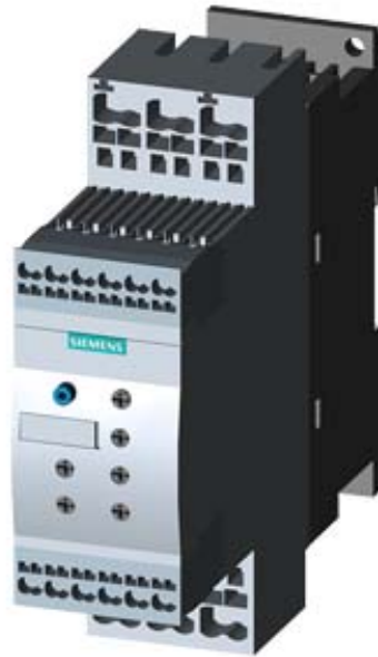
SIRIUS SOFT STARTER, S0, 25A, 11KW/400V, 40 DEGR., AC 200-480V, AC/DC 110-230V, SPRING-LOADED TERMINALS
