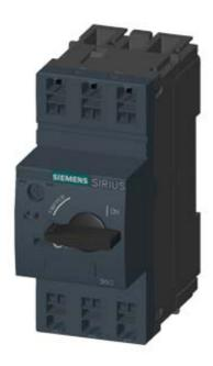
CIRCUIT-BREAKER SZ S00, FOR MOTOR PROTECTION, CLASS 10, A-REL.2.2...3.2A, N-RELEASE 42A, SPRING-L. CONNECTION, STANDARD SW. CAPACITY
