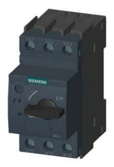
CIRCUIT-BREAKER SZ S0, FOR MOTOR PROTECTION, CLASS 10, A-RELEASE 30...36A, N-RELEASE 432A, SCREW CONNECTION, STANDARD SW. CAPACITY,
